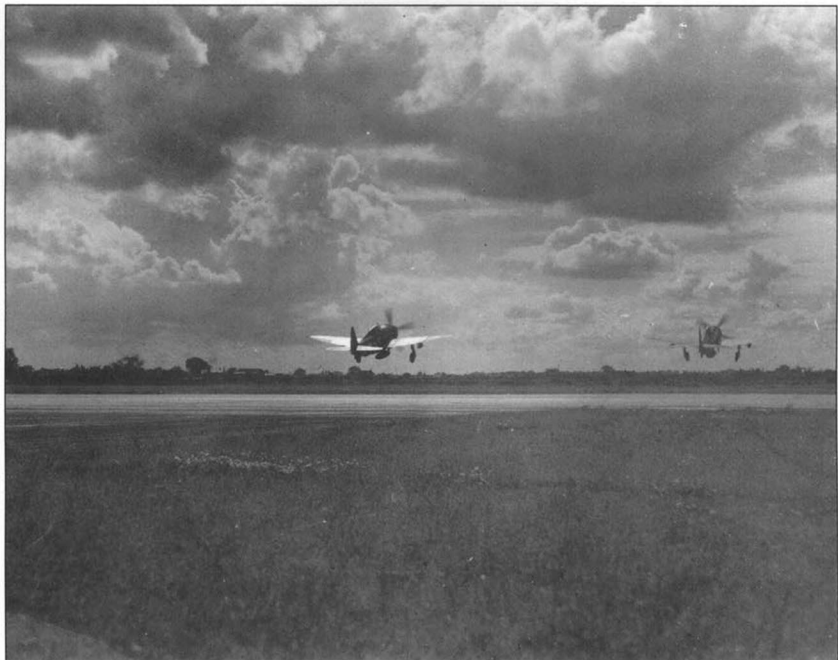
Two 63rd FS Thunderbolts lift off from Boxted's runway 28 for a fighter-bomber mission on the afternoon of 15 July 1944. They are carry 500-lb GP bombs on the wing racks and a 108-US gallon tank under the fuselage
